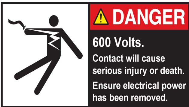
Figure 8 – Danger sticker applied to High Voltage LRUs
